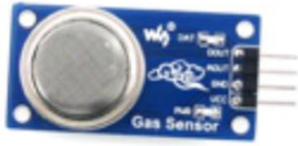
Fig .4 MQ-2 sensor [4]
