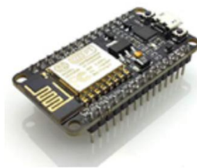
Fig .2 NodeMCU ESP 8266 [7]
