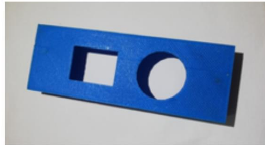
Fig .5 3-D printed enclosure of devices
